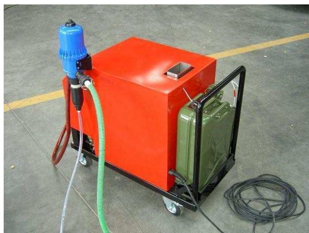
Flow-type heater with chemistry feeder (blue tank)
