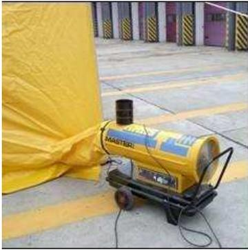
14.5 kW heater connected to NPA tent
