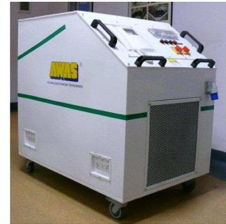
Filter-decontamination machine with HEPA and UV filters
